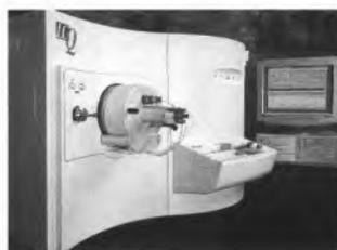
**F2. Novo HPLC com Espectrometria de Massa "Ion Trap" Finnigan - Modelo LCQ**
